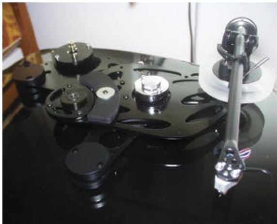
Unique Resolution subchassis (with Expressimo Mongoose tonearm) showing bearing housing and three point suspension.
